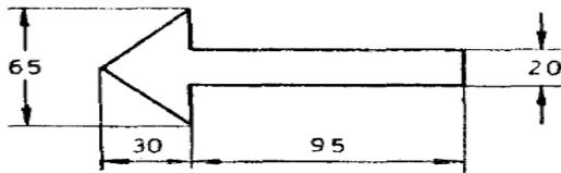
**6A For Pipes DN 200 and Below**
