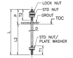
TYP ANCHOR BOLT DETAIL
